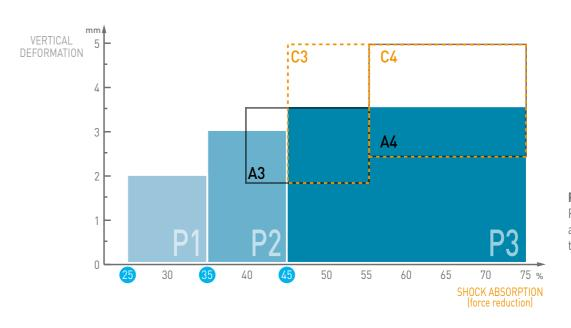
P1, P2, P3: Point-elastic floor shock absorption classes as per the European Standard
